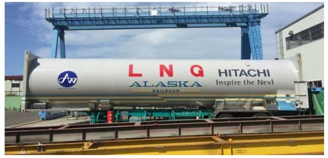
This photo illustration shows a 40-foot cryogenic container that will carry liquefied natural gas at 260 degrees below zero — with an inner and outer steel tank like a thermos bottle. The container was photographed in Japan in August. (Shuji Manabe / Hitachi High-Tech AW Cryo)
